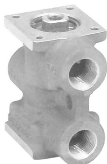
501AA 501AA-3-10-21 Model 501AA is a 3-way or "detented" 3-way, normally closed valve with an internal compensating orifice which maintains actuated position after momentary pilot signal, maintains "trapped" pilot pressure to compensate for minor leaks, and speeds the opening and closing response time. See further information in introductory material about piloted valves.
