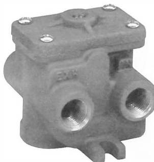
501-4A Model 501-4A valve offers high flow rates (to 212 scfm at 125 psig). With all ports on the same horizontal plane, it provides convenient straight-line plumbing. The 501-4A can be mounted in any position: in-line or with body mounting lugs.
